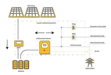
Hybrid inverter will not only provide power to the backup load connected but also give power to the home load connected. If PV power and battery power is insufficient, it will take grid energy as supplement. The hybrid inverter will not sell power to grid. The external CT(&Meter) will detect power flowing back to the grid and will reduce the power of the inverter only to supply the local load, charge battery and home load. This control is achieved by:
