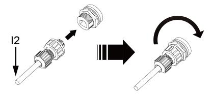
c. Remove the waterproof bridge from DC+ and DC-, then insert the power wire (K2) into DC+ and DC-.
