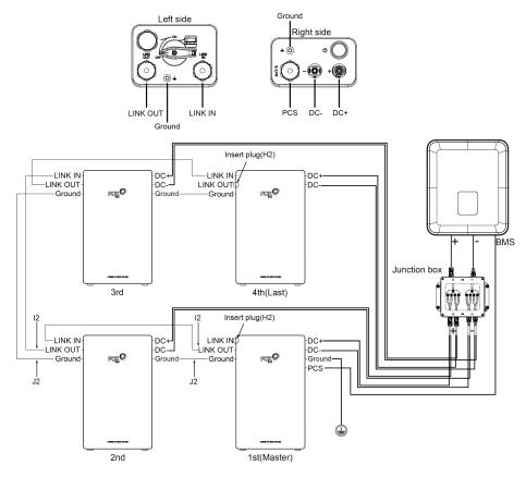
Note: Keep a distance of 300-600mm from the battery to the junction box. Power cable(K2) must be pulled straight from the battery DC+/- for more than 80mm before bending.
