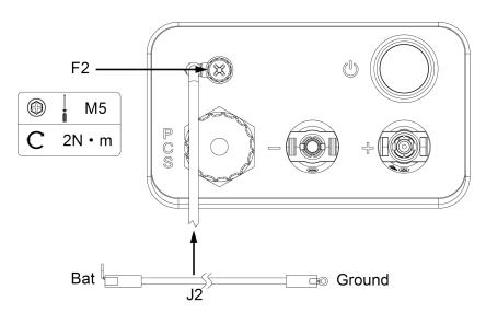
${f b}.$  Connect the PCS communication cable (I2) of the  ${f Master}$  battery to the BMS communication port of the inverter.
