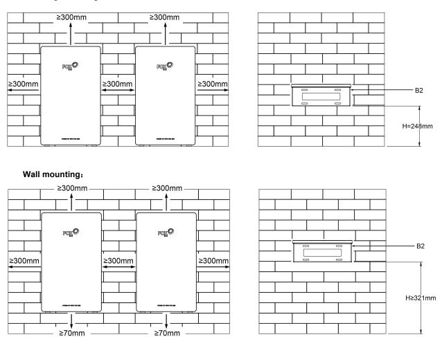
Make sure to leave a space of at least 300 mm. A clearance of at least 300 mm must be left around the battery pack for proper cooling.
