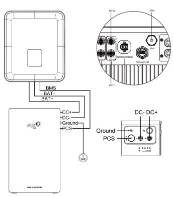
Note: Power cable (K2) must be pulled straight from the battery DC+/- for more than 80mm before bending.
