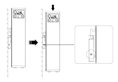
Step 4: Insert 2 pcs of M5\*10 screws (F2) into the holes on the left and right sides of the mounting bracket then tighten the screws.
