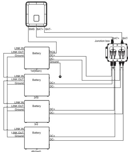
Note: Keep a distance of 300-600mm from the battery to the junction box. Power Cable(L2) must be pulled straight from the battery DC+/- for more than 80mm before bending.
