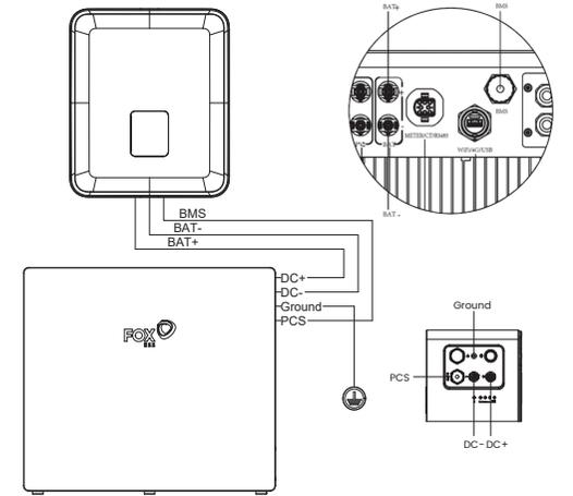
Note: Power Cable (L2) must be pulled straight from the battery DC+/- for more than 80mm before bending.
