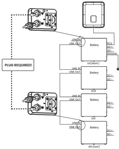
The steps for parallel connection of batteries are as follows:
