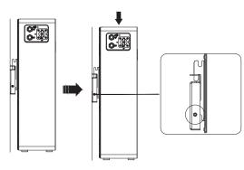
Insert 2 pcs of M5×30 screws (F2) into the holes on the left and right sides of the mounting bracket then tighten the screws.
