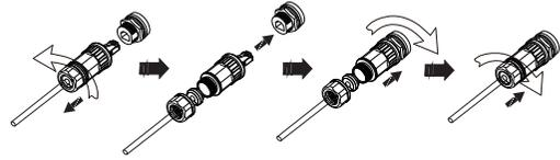
c. Remove the waterproof bridge from DC+ and DC-, then insert the Power Cable (L2) into DC+ and DC-.
