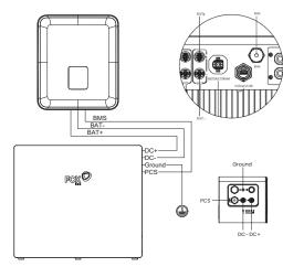
Note: Power Cable (L2) must be pulled straight from the battery DC+/- for more than 80mm before bending.
